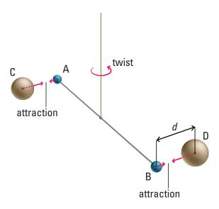
In Cavendish's experiment, the gravitational attraction between the sets of balls caused the fine wire to twist a measurable amount.
